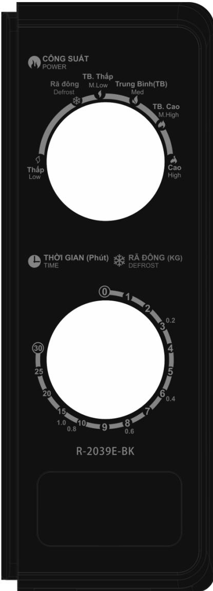
The control panel consists of two function operators. One is a timer knob, and another a power knob.
